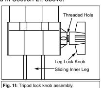
attached equatorial mount (2) to the desired height by loosening the tripod lock knobs and extend the sliding inner section of each tripod leg; then tighten each knob.
